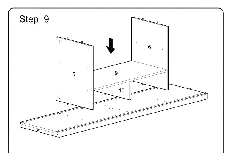
Attach the assembly from the previous step to bottom panel (11) using cam bolts and dowels as guides.
